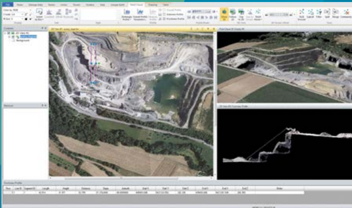
View and edit LIDAR data as well as point clouds created in IMAGINE Photogrammetry and ImageStation.
